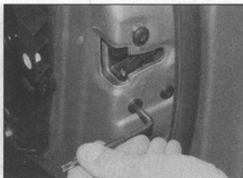
13.13 Unscrew the three door lock screws at the back edge of the door
