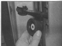
13.10 Unscrew the door wiring harness connector, and push the plug into the door
