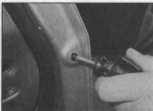
13.4 Remove the handle support screw at the back edge of the door
