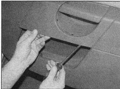
12.4a Prise the door handle trim panel at the base ...
