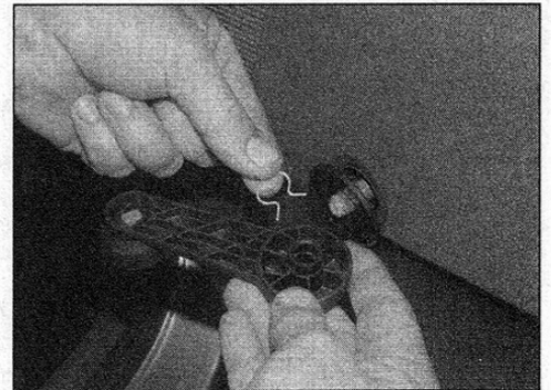
12.12b ... which clips into a groove in the back of the handle
